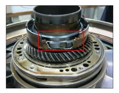
**Photo No. 1**: No. 4 Bearing Key washer from Engine S/N FA0492 exhibiting distress and fracture (*Pratt & Whitney Canada*)
